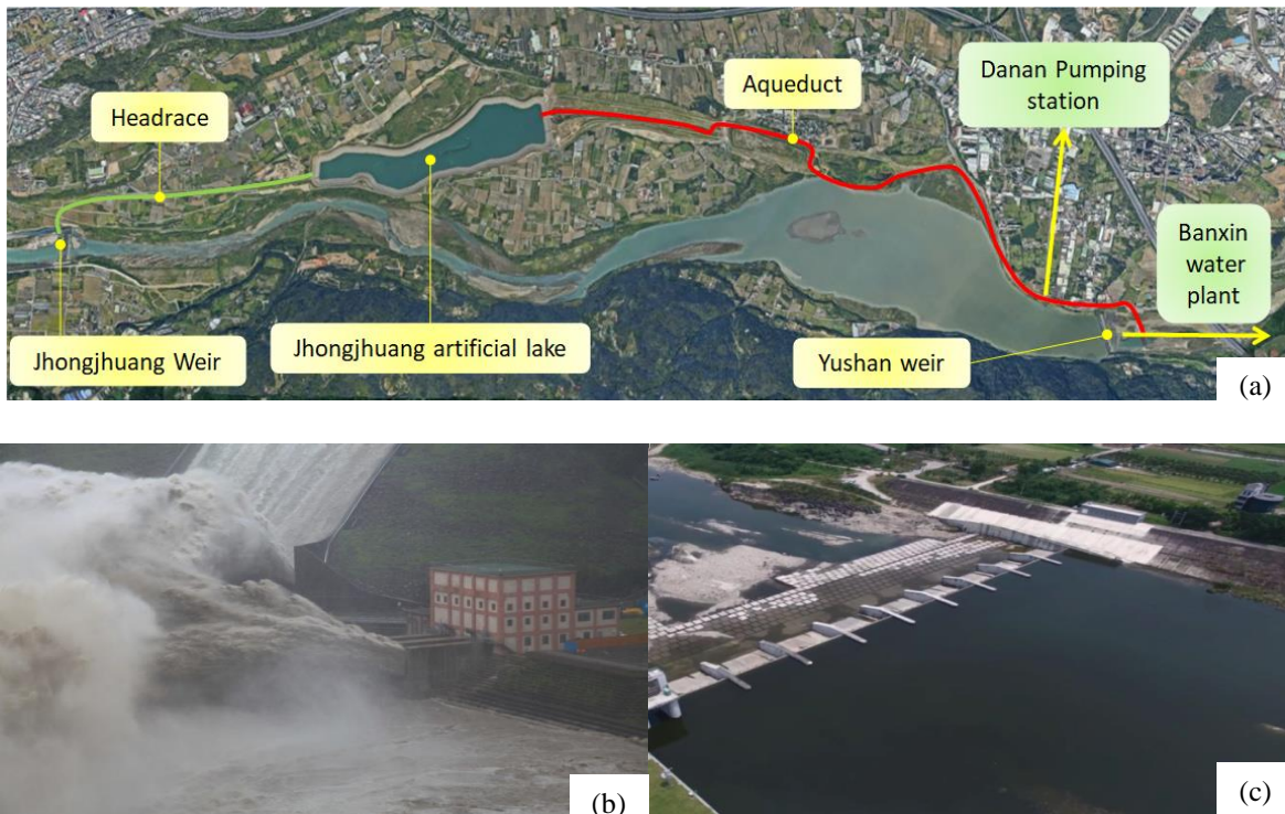
Figure. 3: Pictures of Jhongjuang artificial lake (a) position of Jhongjuang artificial lake (b) sand discharge from desilting tunnel outlet (c) Jhongjuang weir
