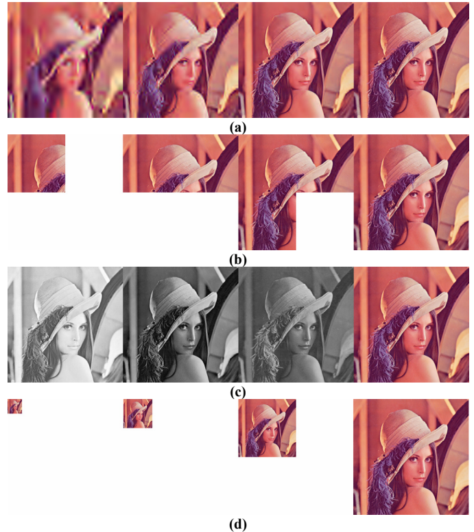
Fig. 1. The four types of progression provided by JPEG 2000: (a) progression by quality; (b) progression by locality; (c) progression by component; (d) progression by resolution.
